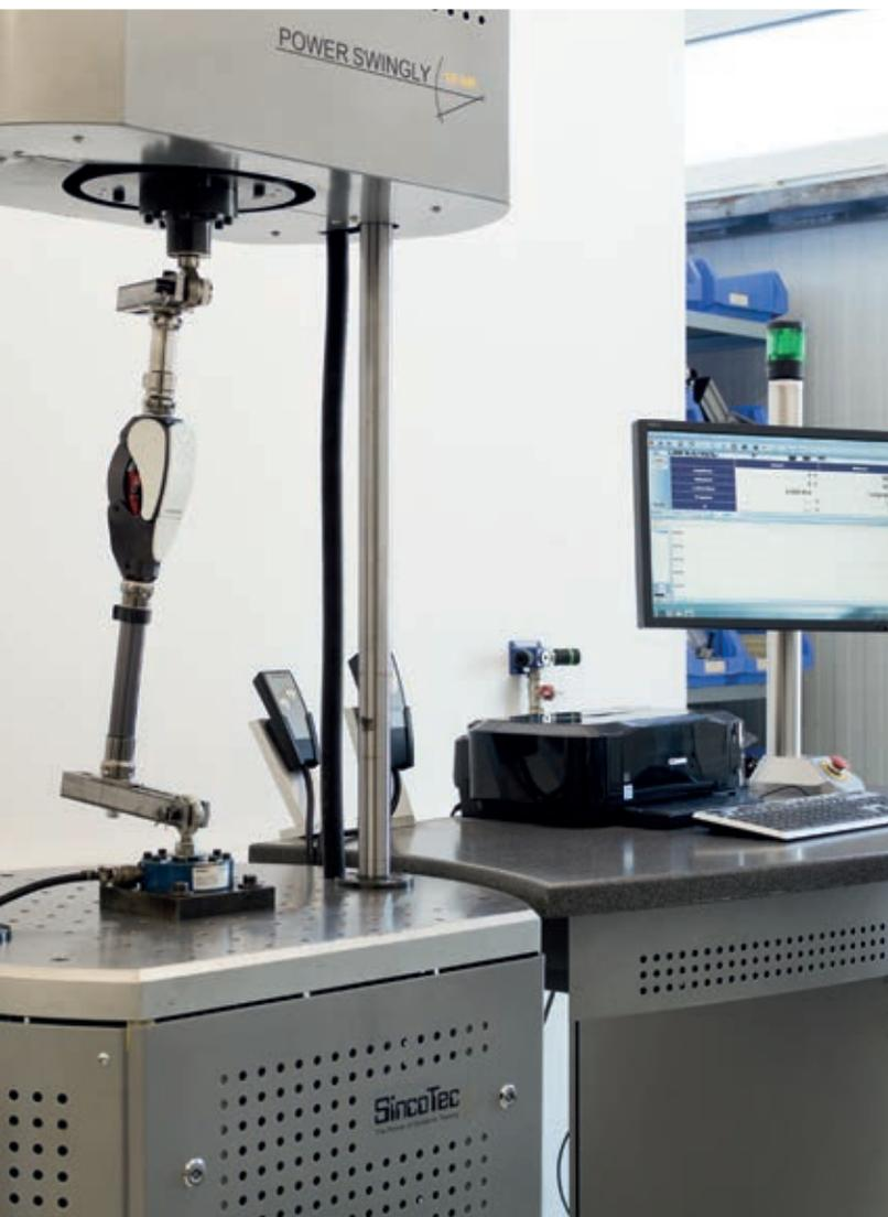
\* Structural testing of lower limb prostheses
